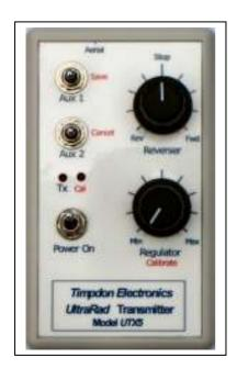
The *UltraRad* Radio Transmitter Model *UTX5* is primarily designed to be used with *UltraRad* Controller Model *URC8* for live steam vehicles. It may, however, also be used with any *UltraRad* radio receiver and controller.
