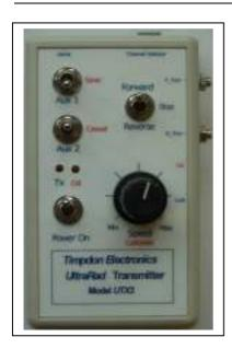
The *UltraRad* Multi-Channel Radio Transmitter Model *UTX3* is designed to be used with any *UltraRad* radio receiver and controller.
