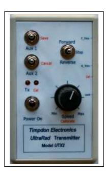
The *UltraRad* Radio Transmitter Model *UTX2* is primarily designed to be used with *UltraRad* Controllers Models *URC3* and U*RC4* for live steam vehicles. It may, however, also be used with any *UltraRad* radio receiver and controller.
