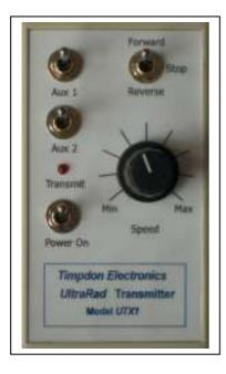
The **UltraRad** Radio Transmitter Model **UTX1** is designed to be used with any **UltraRad** radio receiver and battery electric vehicle controller.
