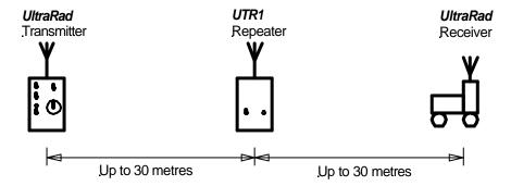
To provide a *fill-in* for shielded areas of your layout, position the repeater where there is direct line of site to both the normal transmitter operating position and the shielded area
