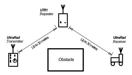
Ideally, the UTR1 repeater should be positioned in open space, a few feet above the ground, with the aerial vertical.
