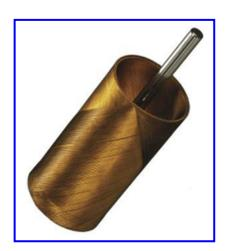
Because the rotating armature is iron free, the moment of inertia is very low, there are no eddy current iron losses, and the armature inductance is very low.
