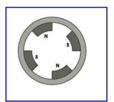
The presence of the heavy iron armature results both in significant eddy current losses within the motor, high moment of inertia, and high motor inductance. The motor efficiency of a small motor rarely exceeds 65% maximum.
