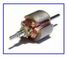
In a standard d.c. motor, the armature comprises a solid laminated iron core, with a number of windings wound in slots along the core. Each separate winding is connected to the commutator and the number of windings represents the number of poles.
