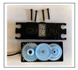
Carefully remove the top case moulding from the top mounting plate by pulling upwards.
