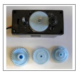
Remove the centre gear only from its bearing. Rotate the output shaft and note that it will only rotate as far as the end stops.
