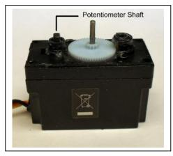
If you have your transmitter available, connect the servo to the channel you will be using to control it, and power up the servo with the output shaft disconnected.
