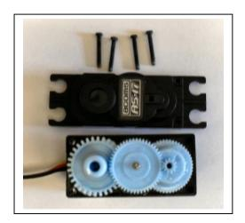
Finally, re-assemble all of the gears on the top plate, refit the top cover and tighten all fixing screws.
