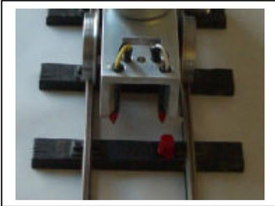
You must ensure that reed switches are positioned so that each switch can be activated only by its own track magnets, and not those associated with the other switch. See below for details of track magnet positioning.
