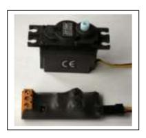
Toggled servo operation with single pulsed trigger switch input.
