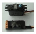
Identical in performance and operation to **SCS1**, but with an additional sense output which switches at the end of servo motion.
