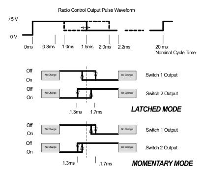
This **RadioSwitch** model is designed to energise one of the two load outputs at any one time and is ideal for the operation of, for example, vehicle head and tail lights, where two separate circuits are required, only one of which is energised.
