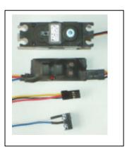
Controlled rotation between two servo positions, with Limit Switch.
