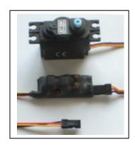
Up – Stop – Down servo control, using centre off joystick.
