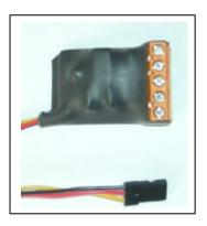
Control four Switches from one RC channel.
