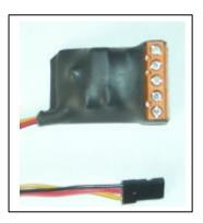
Control four Switches from one RC channel.
