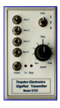
This advanced multi-channel 2.4 GHz GigaRad Radio Transmitter, is designed to be used with any model of GigaRad receiver/ controller.
