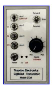
This advanced 2.4 GHz *GigaRad* Radio Transmitter, is designed to be used with any model of *GigaRad* receiver/controller.
