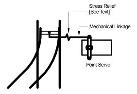
Both the **set** and **reset** positions of the servo are user programmable from the transmitter, operating in a special calibration mode.
