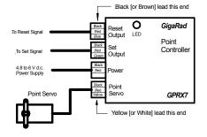
See below for details of connections to auxiliary signal outputs.
