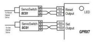
The **Red** and **black** wires supply +5V power to the **SCS1**, and the **Blue** or **Green** wire is the trigger input.
